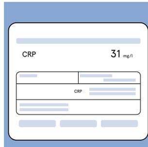
**7** The result appears on the display and the cuvette rises up automatically when the measurement is completed. The QuikRead go CRP+Hb test shows the Hb result below the CRP result.
