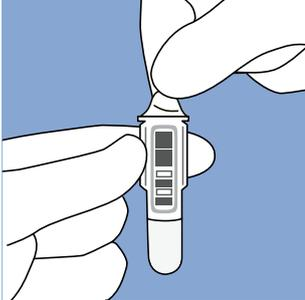
**1** Remove the foil cover from the cuvette. Do not touch the clear flat surfaces in the lower part of the cuvette.
