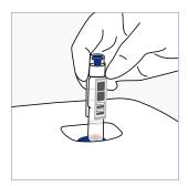
Choose Quality control on the display of the QuikRead go Instrument. Insert the cuvette into the measurement well of the instrument. The barcode should be facing you.
