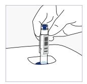
Choose Quality control on the display of the QuikRead go Instrument. Insert the cuvette into the measurement well of the instrument. The barcode should be facing you.
