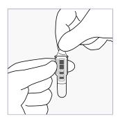
Remove the foil cover from the cuvette. Do not touch the clear flat surfaces in the lower part of the cuvette.
